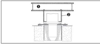
Figure 3.9. Vertical Down Firing Block
