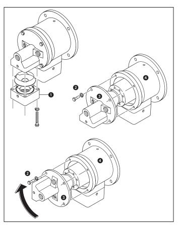
Figure 3.1. Rotate the Rear Cover
