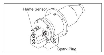
Figure 3.2. Installing the Flame Sensor
