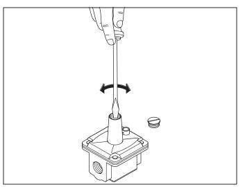
Figure 4.2. Adjusting Ratio Regulator Screw
